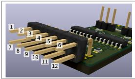
Figure 1: Pin numbers of Pmod connector on host FPGA board and SMA Plug module
